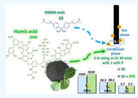
tests, and hence an increase (up to 1.8 min) of the time to flashover, without any detrimental effect on the overall mechanical behavior. The evolved gas, thermal, and fire analysis was used to propose the combined mode of action of HA, UR, APP, and silicon in the fire performance improvement of the hybrid epoxy system.
