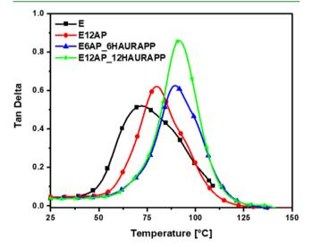
Figure 3. Mechanical damping factor  $(\tan \delta)$  of pristine resin and epoxy composites collected as a function of temperature.
