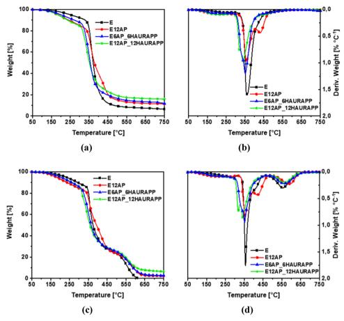
Figure 2. (a, c) TGA curves and (b, d) DTG curves of EPO and epoxy composites under N<sub>2</sub> (a, b) and air (c, d).
