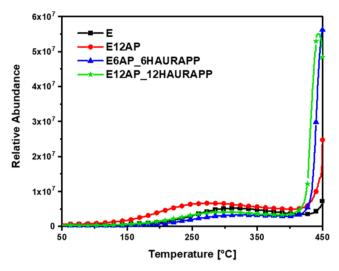
**Figure 8.** DIP-MS total ion thermograms of E, E12AP, E12AP 12HAURAPP, and E6AP 6HAURAPP samples.
