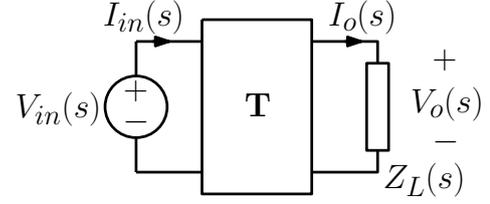
Fig. 5. Equivalent circuit for a  $N$ -modes piezoelectric energy harvester.
