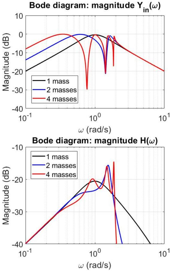
Fig. 6. Bode diagram for the magnitude of the input admittance  $Y_{in}(\omega)$  (above) and the voltage ratio  $H(\omega)$  (below), for the circuits shown in figures 3 and 4. For the sake of simplicity all parameters are normalized to 1, except  $\alpha = 0.5$ .
