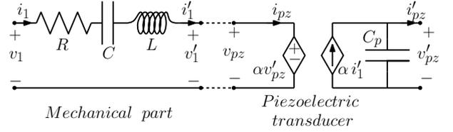
Fig. 3. Equivalent circuit for a single mass energy harvester with piezoelectric transducer.
