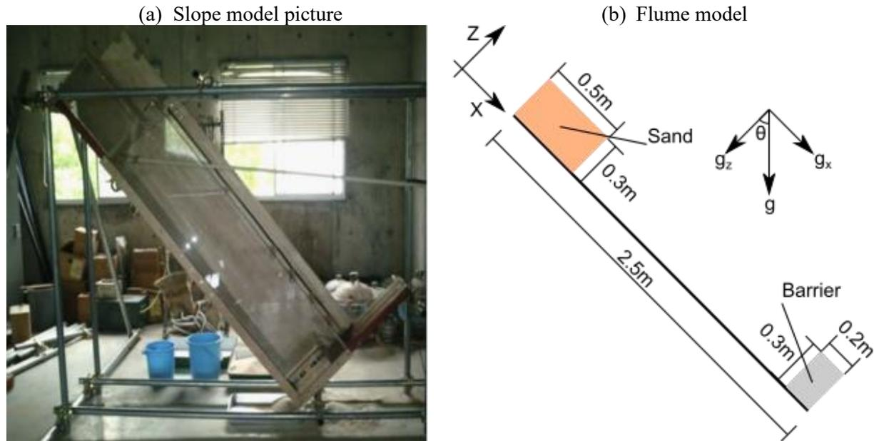
**Figure 1:** Laboratory flume (a) assembled by Moriguchi et al. (2009) and its scheme implemented in the simulations (b). The sand is placed at the top of the flume with slope angle  $\theta = 45^\circ$ . A barrier is placed 1.8 m from the gate.
