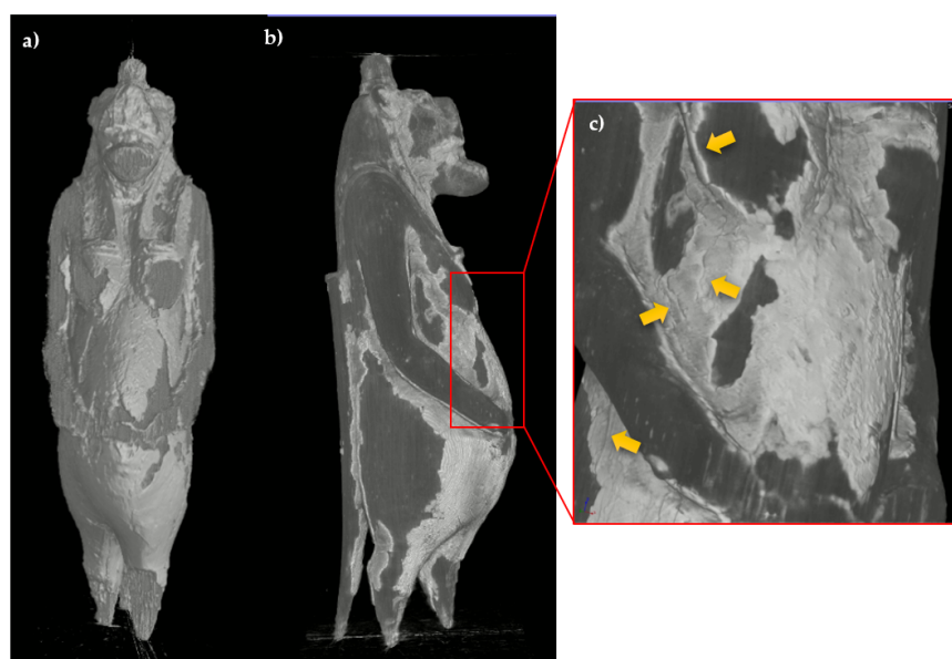
Figure 9. 3D model of the statuette with different surface render tools, ((a), Scatter Gradient v1.2 tool), ((b), Hardware render (scatter gradient) tool); enlargement of the body area in which the cracking is visible (yellow arrows) (c).
