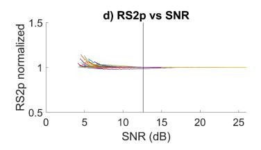
**Figure 5.** Plots of respectively R-S<sub>1,M</sub>, R-S<sub>1,T</sub>, R-S<sub>2,A</sub>, and R-S<sub>2,P</sub> in function of the SNR of the signal for all 25 subjects. All values were normalized with respect to the value corresponding to the highest SNR for the purposes of comparison. The black vertical lines represent the computed minimum acceptable SNR values. Each colored line represents a subject from the sample population.
