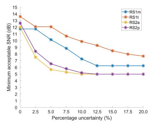
**Figure 6.** Minimum acceptable SNR for the estimation of respectively  $R-S_{1,M}$ ,  $R-S_{1,T}$ ,  $R-S_{2,A}$ , and  $R-S_{2,P}$  as a function of the acceptable percentage uncertainty over the measurement of the hearth valves closure latencies.
