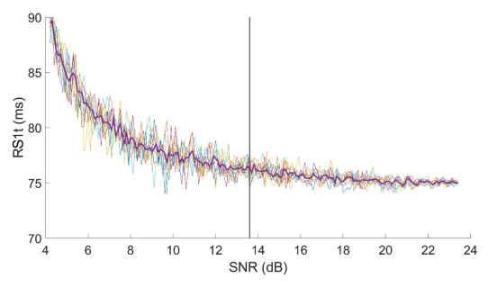
**Figure 4.** Example of R- $S_{1,T}$  variation in function of the SNR of the signal. Each colored line represents a different test on the same signal. The thicker violet line represents the median, which is taken as representative for the signal. The vertical line represents the minimum SNR value considered as acceptable.
