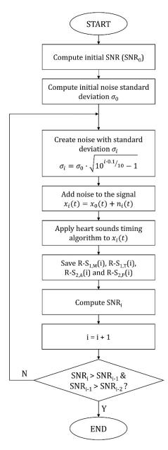
**Figure 2.** Flowchart of the algorithm described in this work.  $R-S_{1,M}$ ,  $R-S_{1,T}$ ,  $R-S_{2,A}$  and  $R-S_{2,P}$  are the latencies of the mitral, tricuspid, aortic and pulmonary valves with respect to the corresponding R-peak.
