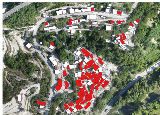
Figure 4. The image shows the damage classification performed by DEEP on the Pescara del Tronto 2016 orthophoto, using the Mozambique classification model. The not-affected buildings are marked in white, while the damaged buildings are marked in red colors.
