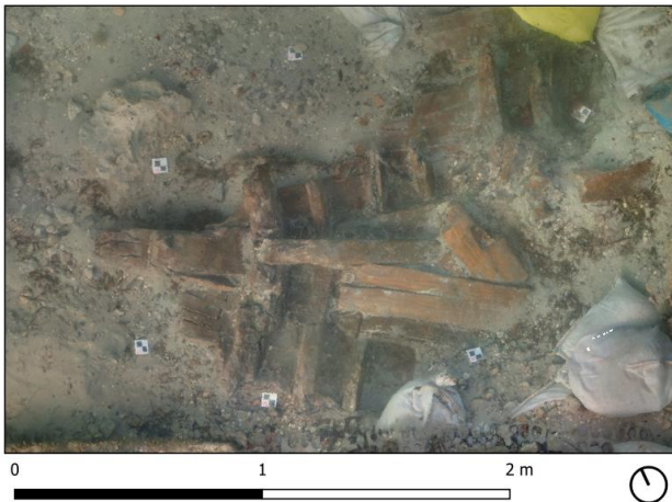
Figure 9. Orthoimage of the aft part of the shipwreck, georeferenced using five 10 cm squared checkerboard markers, measured with celerimetric method.
