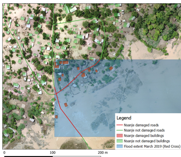
Figure 9. UAV orthophoto of Nsanje (UNICEF 2019); superimposed the flood extent layer (blue) with the affected buildings and roads (in red) after the 2019 Cyclone Idai flooding.
