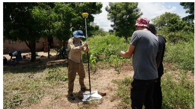
Figure 4. GCPs measurements in Nsanje district.
