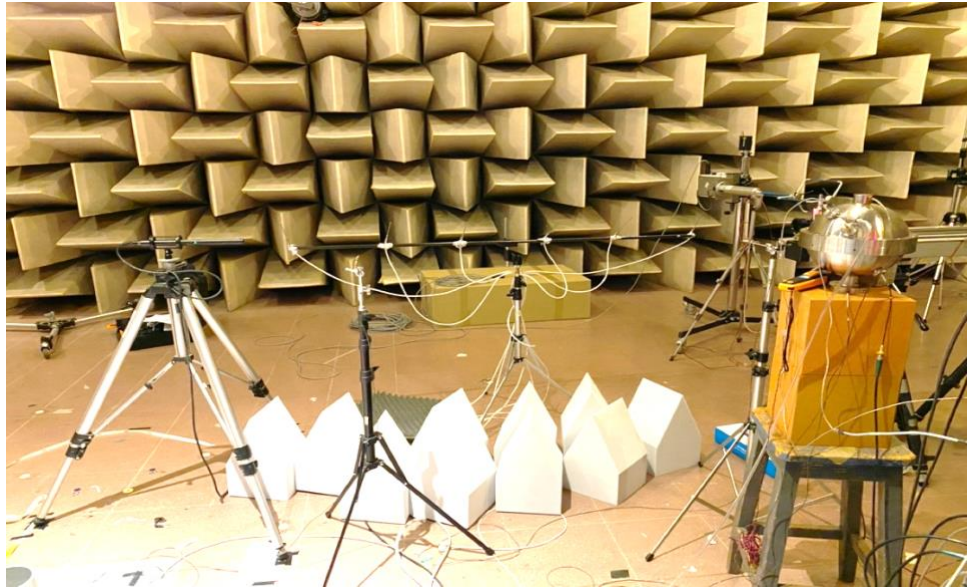
Figure 48-Foams between loudspeaker and microphone at original position
