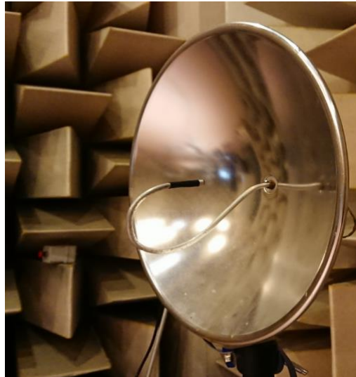
Figure 9- Some of the microphones and loudspeakers used in the preliminary study for the experiment. Above: a horn loudspeaker and a loudspeaker placed in the focus of a parabolic reflector. Below: an interference super-cardioid microphone and an omni-directional microphone placed in the focus of a parabola.
