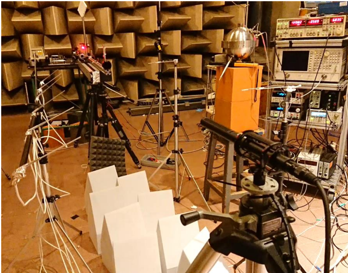
Figure 23-Experimental set-up for the measurement of the speed of sound. At the background/left is visible the carriage carrying the loudspeaker. At the foreground on the right is visible the microphone on the tripod. At the left the array of resistance thermometers. Top right the experiment with the spherical resonator. On the floor foam absorbers for reducing acoustic reflections
