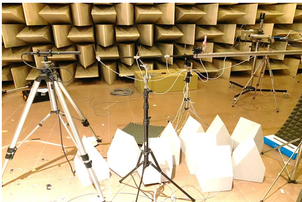
Figure 49- Foams between loudspeaker and microphone at re-arranged position
