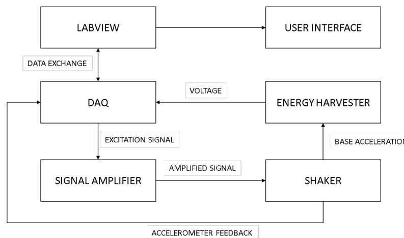
**Figure 5.** Input/output scheme of the experimental apparatus.
