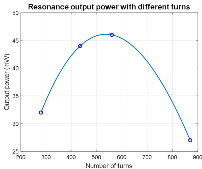
Figure 19. The optimum power with respect to the number of turns.
