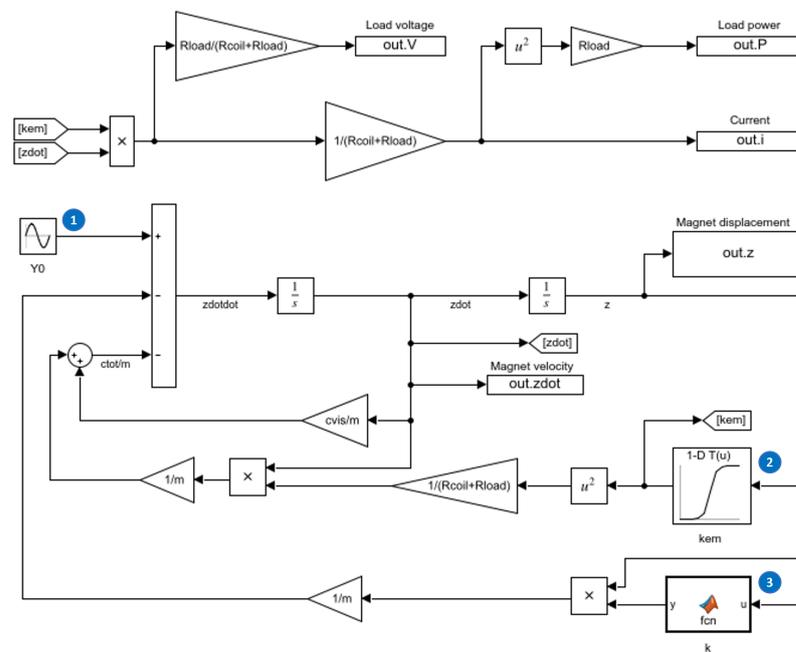
Figure 8. Simulink model of the energy harvester.
