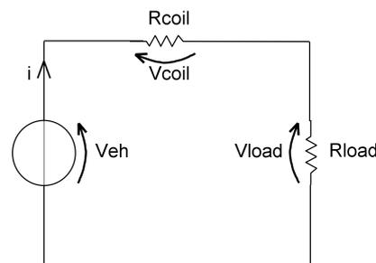
Figure 11. Electrical circuit of the energy harvester.
