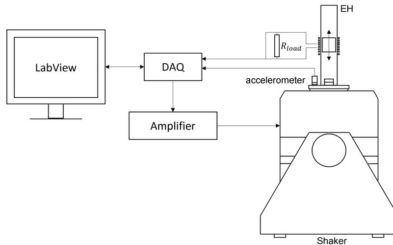
Figure 6. Input/output scheme of the experimental apparatus.
