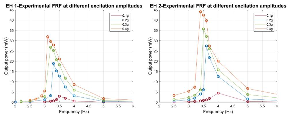
**Figure 14.** Experimental RMS power FRF for different excitation amplitudes, on the left, for EH 1 and, on the right, for EH 2.
