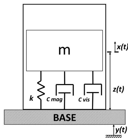
Figure 7. The 1 d.o.f mass–spring–damper scheme model.
