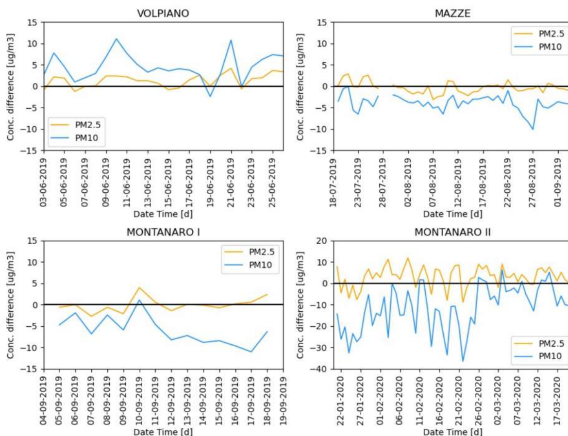
Figure 5. Differences between the data acquired by the two APM-2s in the external sites and the fixed urban station located in Politecnico di Torino (Turin, Italy). An almost null trend for PM_{2.5} delta was obtained. The PM_{10} trend was affected more by the local situation. PM_{10} suburban station values were generally lower than the fixed one, but the Volpiano campaign presented an opposite trend because of boundary conditions.
