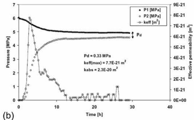
Fig. 5 – Residual capillary pressure procedure (a) and results of a lab test (b) (Hildenbrand et al, 2002 and (Hildenbrand et al, 2004).
