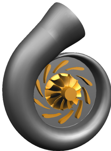
Figure 1.6 Variable Geometry Turbine components: volute, vanes, rotor. Courtesy of General Motors.
