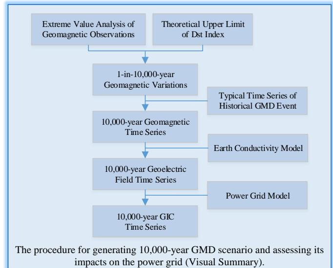
In this study, we model the 10,000-year GMD event using the extreme value analysis and then assess the GIC in the power grid. Although located at low latitudes, the 1000 kV Sanhua UHV power grid with long transmission lines and small DC resistances may be subjected to large GIC levels [8]-[9]. For illustration, a case study of the 1000 kV Sanhua UHV power grid under 10,000-year GMD scenario is carried out.
