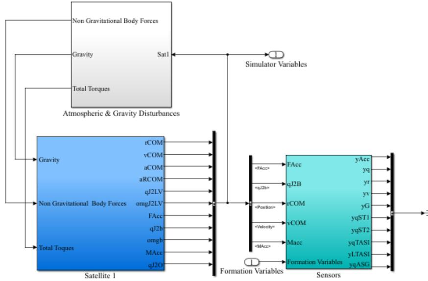
Fig. 1. Nonlinear Model of a Single Satellite
