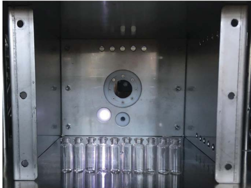
Figure A1. Picture of the box used with the IR sensor behind it and 10 vials placed ~25 cm from the sensor, as set for the experiments. The front wall of the box was removed for the picture.
