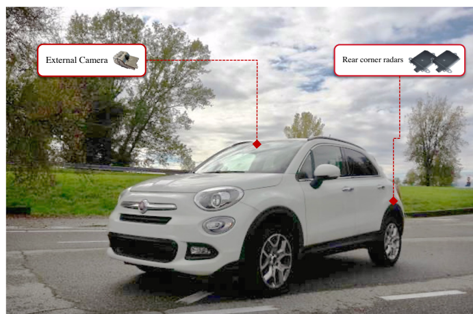
Figure 2. Prototype vehicle with installed sensors.
