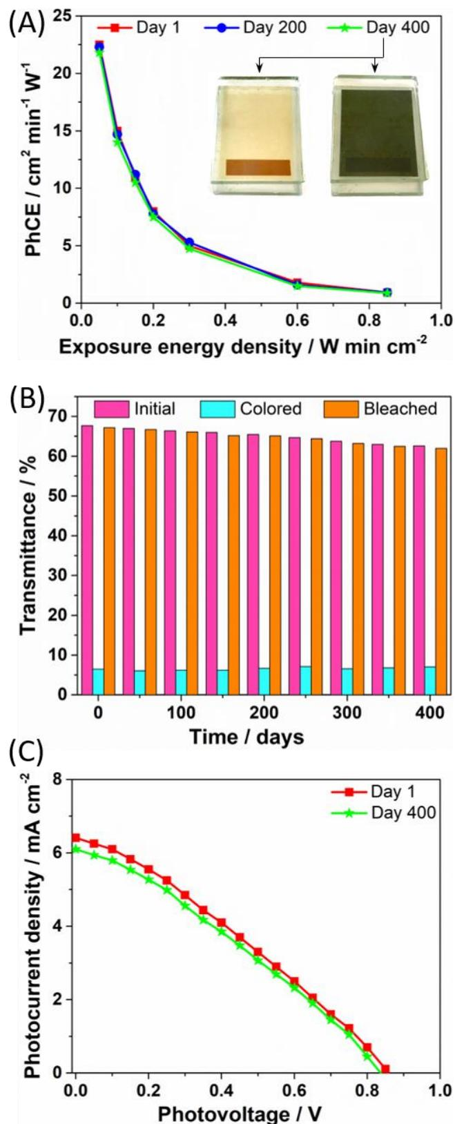
**Fig. 4.** (A) PhCE of the PECD under 1 sun irradiation, comparing the values calculated at day 1, day 200 and day 400 of the ageing test. The inset shows pictures taken at day 400 under colored and bleached conditions, respectively. (B) Luminous transmittance vs. ageing time for the PECD. (C) J–V curves of the DSSC portion of the PECD, measured under 1 sun irradiation (AM1.5G) just after fabrication and at day 400 of the ageing test.
