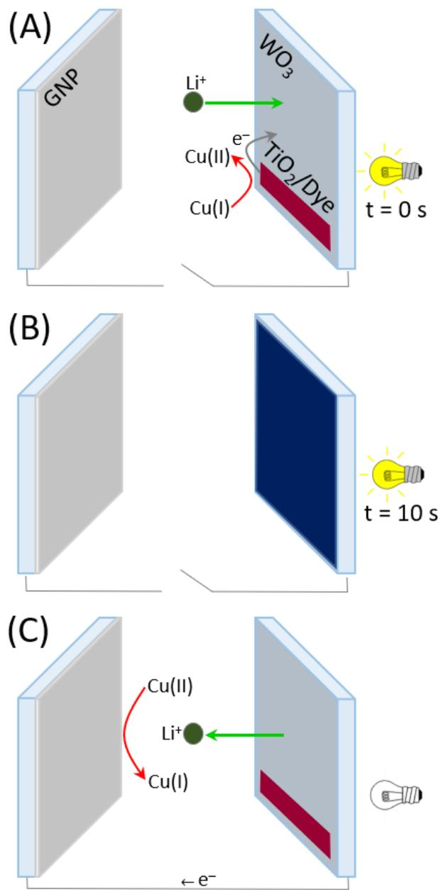
**Fig. 2.** Schematic diagram of the PECD in: (A,B) open-circuit conditions under simulated sunlight (at  $t = 0$  and after 10 s); (C) short-circuit under dark conditions. The oxidation and reduction of the Y123 dye is not drawn so as not to complicate the readability of panels (A) and (C).
