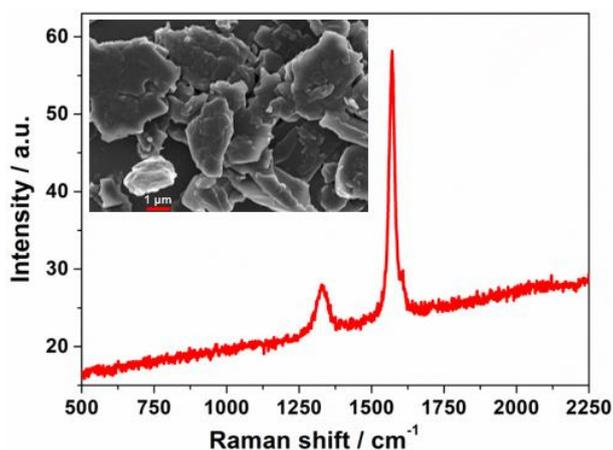
**Fig. 1.** Raman spectrum of GNPs used as CE material. *Inset:* FESEM micrograph of GNPs onto the PECD conductive glass, just after deposition and solvent evaporation.
