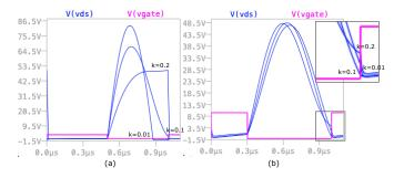
Fig. 3. Spice simulations of the proposed designs showing ZVS or quasi-ZVS for three different values of the coupling factor:  $k=0.01,\,k=0.1$  and k=0.2. (a): voltage across the MOS with respect to the gate control voltage according to the classical approach. (b): voltage across the MOS with respect to the gate control voltage according to the alternative approach. The top right square box represents a zoom at the clock edge to better distinguish the waveforms.
