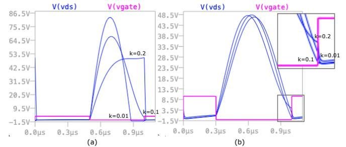
Fig. 3. Spice simulations of the proposed designs showing ZVS or quasi-ZVS for three different values of the coupling factor:  $k = 0.01$ ,  $k = 0.1$  and  $k = 0.2$ . (a): voltage across the MOS with respect to the gate control voltage according to the classical approach. (b): voltage across the MOS with respect to the gate control voltage according to the alternative approach. The top right square box represents a zoom at the clock edge to better distinguish the waveforms.
