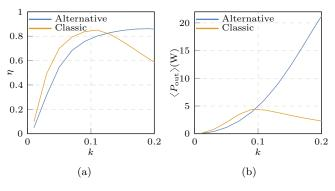
Fig. 4. Comparison of the performances between the two class-E DC-DC converter design methodologies against coupling factor variation. (a): efficiency of the converter calculated as  $\langle P_{\rm out} \rangle / \langle P_{\rm in} \rangle$ ; (b): power absorbed by a resistive load  $R_L = 50 \,\Omega$
