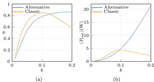
Fig. 4. Comparison of the performances between the two class-E DC-DC converter design methodologies against coupling factor variation. (a): efficiency of the converter calculated as  $\langle P_{out} \rangle / \langle P_{in} \rangle$ ; (b): power absorbed by a resistive load  $R_L = 50 \Omega$
