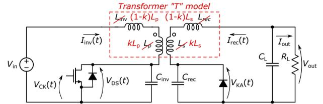
Fig. 2. Schematic of the isolated class-E DC-DC converter (black color) and the modification (red color) derived from the novel approach. The low- $k$  transformer leakage inductances are exploited to avoid extra components.
