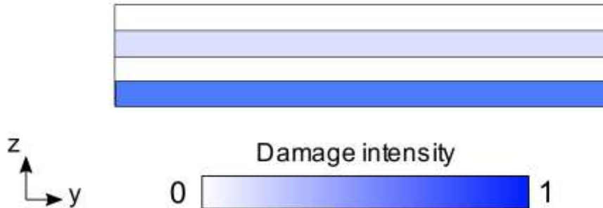
Figure 1. Example of damage introduction in a four-layer plate.
