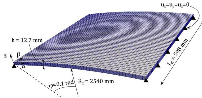
Figure 4. Representation of the VAT curved panel.
