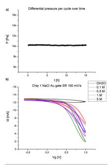
Figure 2. a) pressure reached at each cycle over time b) transfer characteristics of OECT in NaCl with different concentrations, Au gate electrode.
