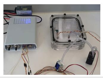
Figure 1. System assembled: electronic dedicated control unit (left), culture chamber (right).
