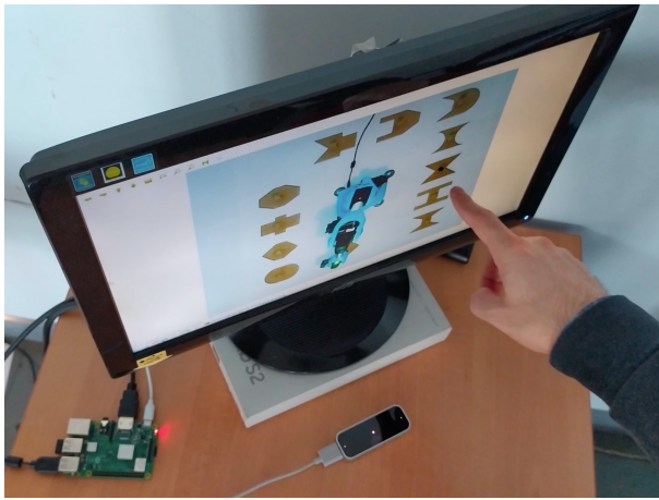
(a) The human operator point-taps the second piece for assembly.
