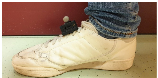
Fig. 1. Experimental setup: a retro-reflective marker is attached on the MIMU which is fixed to shoelaces of each foot.
