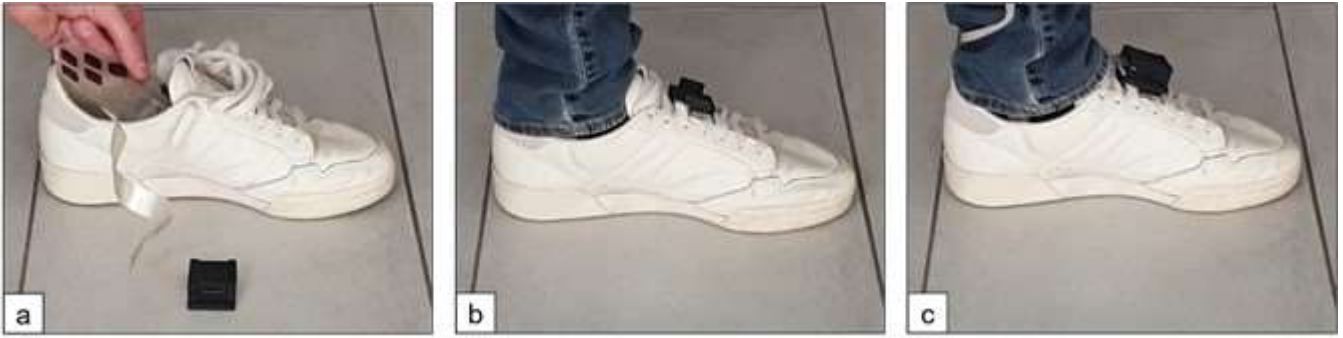
Figure 3: a) PI positioning inside the shoe; b) Clip attached to shoe laces; c) Final sensors positioning with magneto-IMU fixed to the clip.
