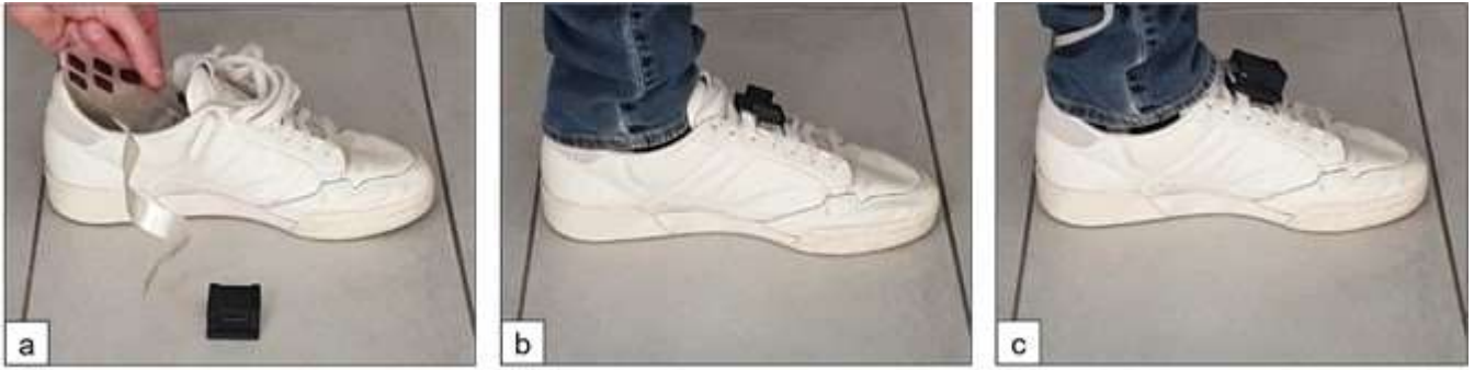
391 392 Figure 3: a) PI positioning inside the shoe; b) Clip attached to shoe laces; c) Final sensors positioning with 393 magneto-IMU fixed to the clip. 394 395
