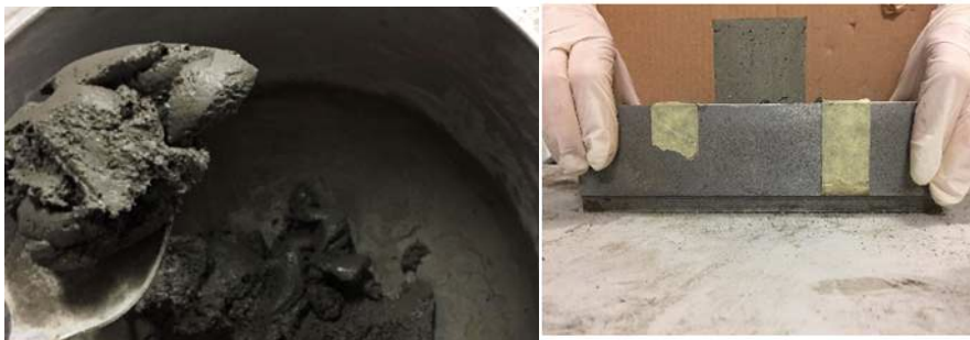
Fig. 2. Representative photograph of the high consistency of the mortars with biochar additions (left) and extrusion test to assess the suitability for 3D printing applications (right).
