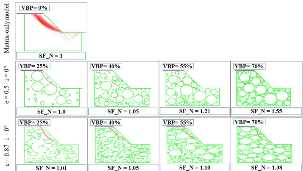
**Fig. 7** Superimposition of the 15 failure surfaces obtained for each VBP considered from the bimrock configurations having blocks with  $e=0.5$  and  $i=0^\circ$  and  $60^\circ$ . The matrix-only model result is also shown with the dotted line, by way of comparison
