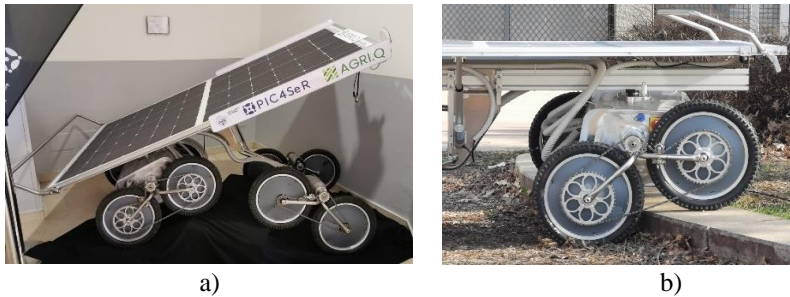
Fig. 1. a) Agri.q in a simulated rough terrain condition: the wheels system adopted allows a force distribution similar so that of a tracked vehicle; b) filter with respect to the oscillations.
