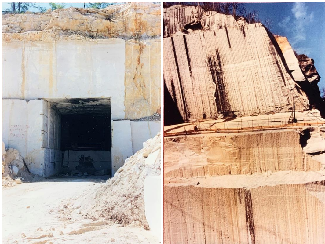
Figure 3. Left: underground voids in hard limestone obtained by cutting saw (Croatia). Right: dynamic splitting in granitic rock for dimension stone quarrying (Italy). Both cases represent good results in terms of stability and block recovery ratio. (credits Oggeri)
