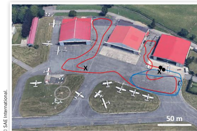
FIGURE 4 Aerial views of the driving scenario (experimental tests). Intended paths for the retained racing prototype (red) and compact SUV. Start of the track (black cross), end of the track (black dot). The actual path can vary, as it is not perfectly reproducible.
