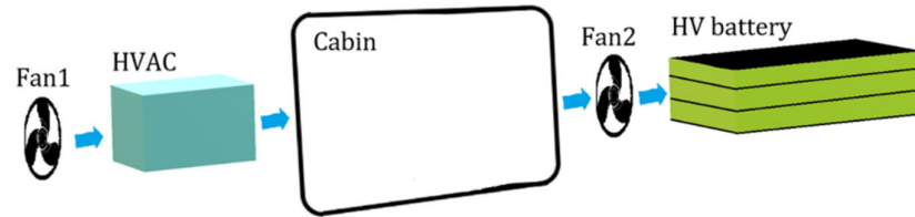
Figure 4. Schematic diagram of the cabin and battery air cooling system.
