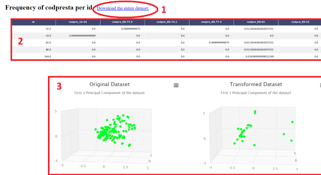
Figure 5: Layout that illustrates how the page showing each transformation obtained is divided. In rectangle 2 the first five lines of the new dataset are shown, while clicking in the red circle at the top the user can download the entire dataset in csv format. Finally, in rectangle 3 there is the comparison between the 3d distribution of the dataset before and after the transformation
