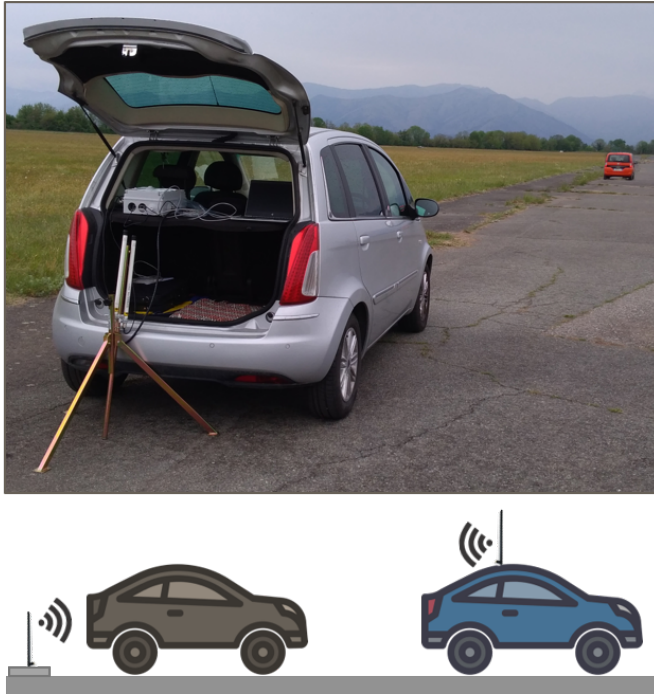
Figure 1: Test setup for measurements under NLOS conditions.
