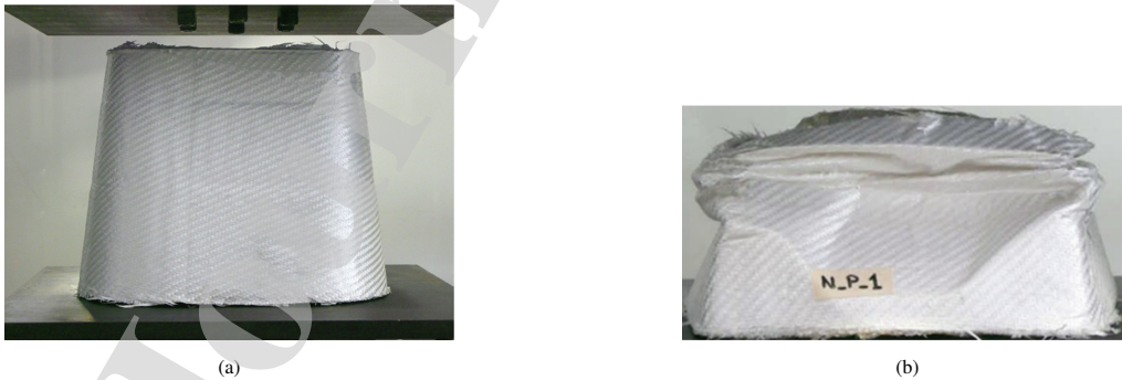
Figure 2: Crush test set- up (a); Impact attenuator after crushing test (b).
