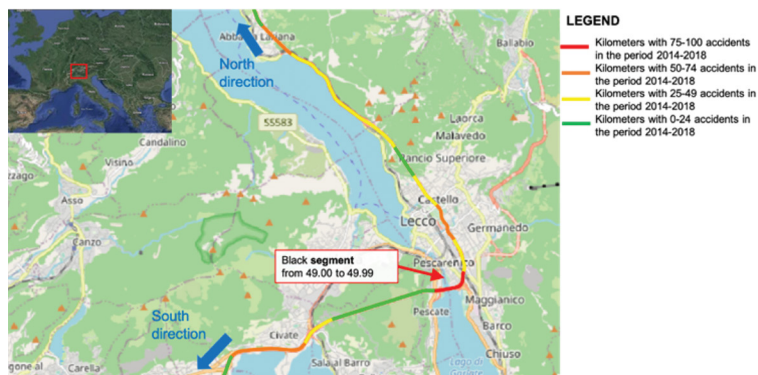
Figure 3: Coloured-scale representation of the critical segments (zoom of the scratch of the State Road 36 where they are localized). Source: www.openstreetmap.org.
