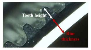
Figure 4. Double-arc profile of the flexspline tooth.
