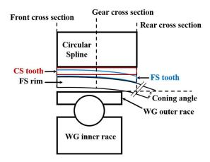
Figure 6. Uneven engagement between flexspline and circular spline caused by the coning angle.
