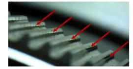
Figure 9. Flexspline tooth cracks.
