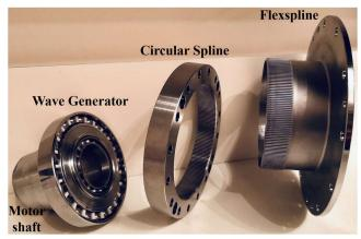
Figure 3. Main components of a harmonic drive gear.
