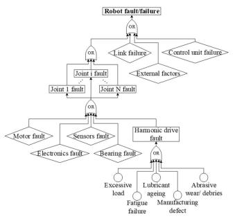
Figure 2. Robot arm fault tree analysis.
