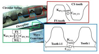
Figure 10. Schematic representation of the contact models used for the different interfaces in the harmonic drive.
