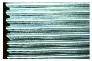
Figure 7. Pitting of the flexspline teeth detected on the shoulder joint of a UR5 collaborative robot.
