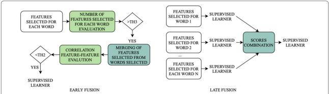
**Fig. 3** Comparison between early and late fusion approaches: in the first case, the features derived from each word are joined before performing the supervised learning; in the second one, separate scores are learned for each word, joined, and used as input of a second supervised learning step
