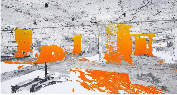
Figure 14. Virtual visualisation of the point clouds within Unreal Engine 4. Orange gradient: SfM; Greyscale: LIDAR
