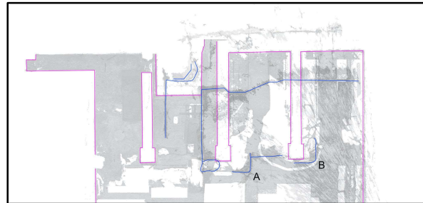
Figure 10. Vector drawing. Purple: underground areas of the basilica (accessible nowadays). Blue: retracing of the SfM point cloud. A and B: foundation pilasters.
