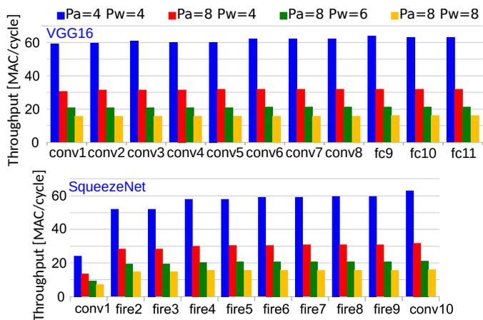
Fig. 4. Layers throughput over several bitwidth combinations.
