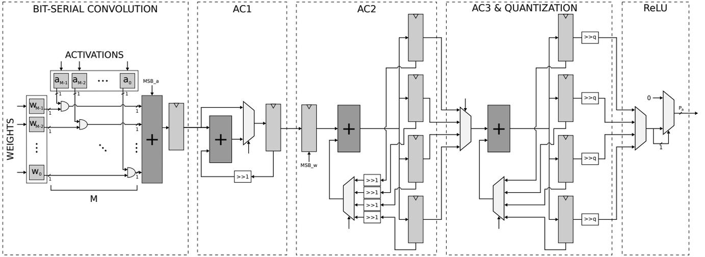
Fig. 2. Datapath architecture of a single SMAC block.
