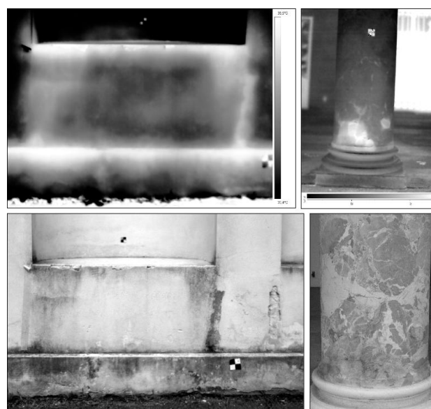
Figure 7. East façade (left), and main façade left column (right) anomalies observed by thermographic imaging and principal component analysis of the multiband data (first components).
