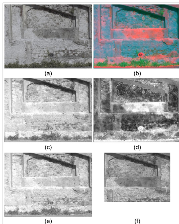
Figure 6. Castello del Valentino riverside façade multiband results: (a) cropped VIS image; (b) TIR-NIR-red false-color composite; (c,d) principal component analysis—first and second component; (e) Fourier transform; (f) quantized image.
