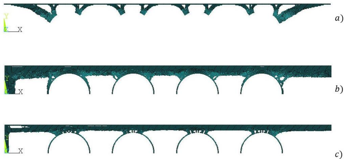
Figure 15 – Final material distribution after: a) fully thermal topology optimisation, b) fully structural topology optimisation, c) thermo-mechanical topology optimisation.
