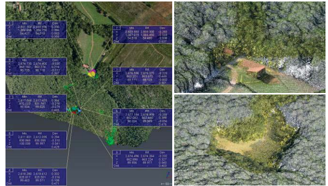
Fig.4. The process of co-registration between the georeferenced UAV DSM and the SLAM-based scans, supported by the common areas where the visibility is allowed both from the aerial and the terrestrial view
