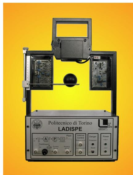
Figure 10. Magnetic levitation system.
