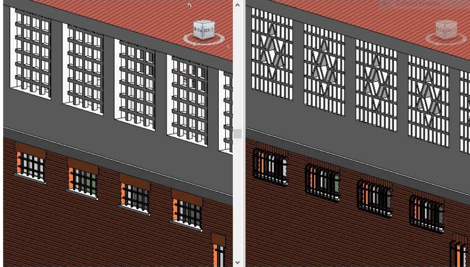
Fig. 12. Details of the colombarius, reconstruction from the design drawing and the photos of realized building. (BIM Modelling: F. Natta).
