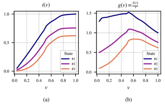
Fig. 2. (a) Average, normalized  $i/v$  characteristics of PCM in three different states. The curves have all been normalized with respect to the maximum current in state #1,  $I_0$  ( $i = I/I_0$ ). The applied voltages have been normalized as well with respect to the maximum applied voltage  $V_0$  ( $v = V/V_0$ ). (b) Large-signal, normalized conductance  $g = i/v$ .
