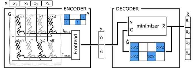
Fig. 1. Architecture of a PCM-based system for CS applications with the proposed decoder. The encoder implements the ideal, binary sensing matrix  $A$  by PCM conductances. The decoder reconstructs the original signal by iteratively computing the estimate of the real sensing matrix  $\hat{G}$ .
