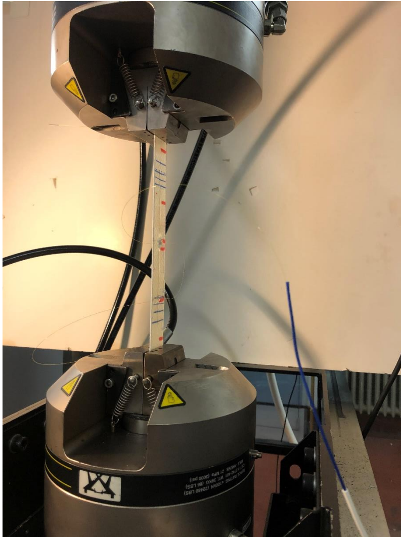
Figure 5.10 Tensile test of specimens equipped with optic fibre.
