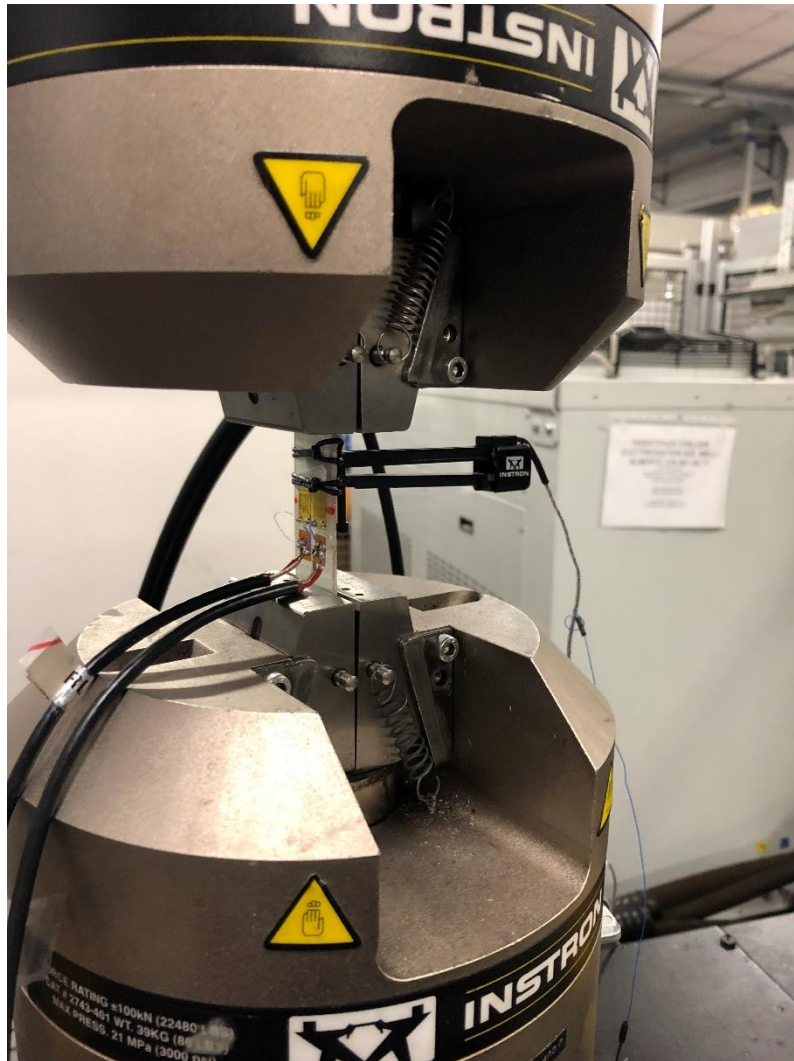
Figure 5.2 Experimental setup of the tensile tests.
