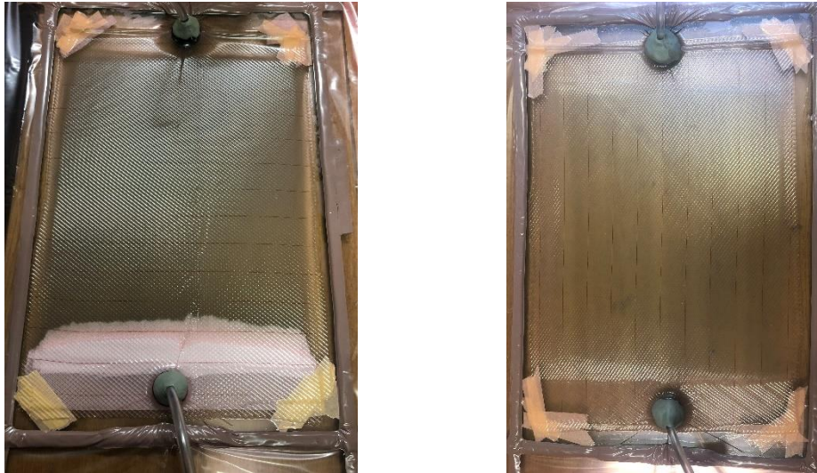
Figure 5.1 Vacuum bag infusion process.
