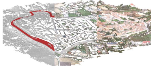
Figure 2. Urban scale cloud segmentation. From the left: DSM and DTM point cloud segmentation, road detection based on radiometric values.
