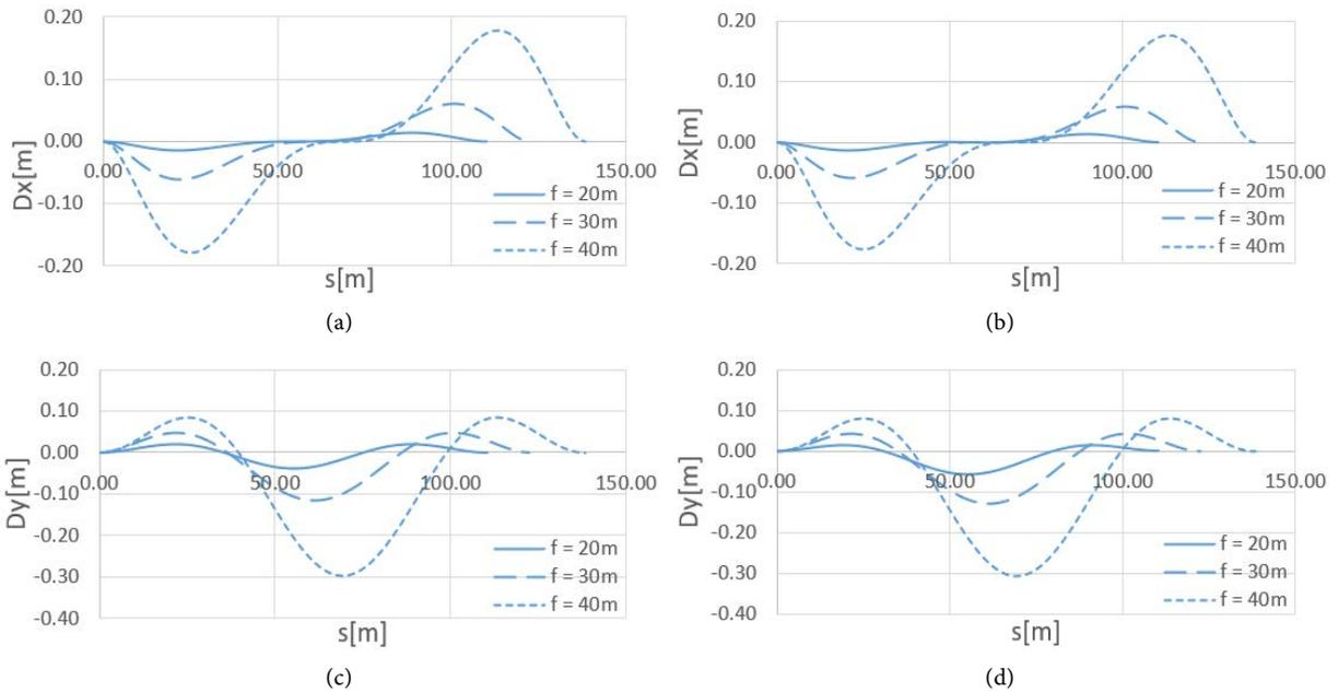
**Figure 3.** Comparison of the Displacements in the global coordinate system ( $x, y$ ): Displacements in the  $x$ -direction (MATLAB (a) and Midas (b)), Displacements in the  $y$ -direction (MATLAB (c) and Midas (d)).
