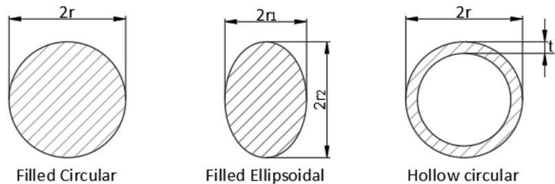
**Figure 7.** Geometrical parameters of the cross-sections.
